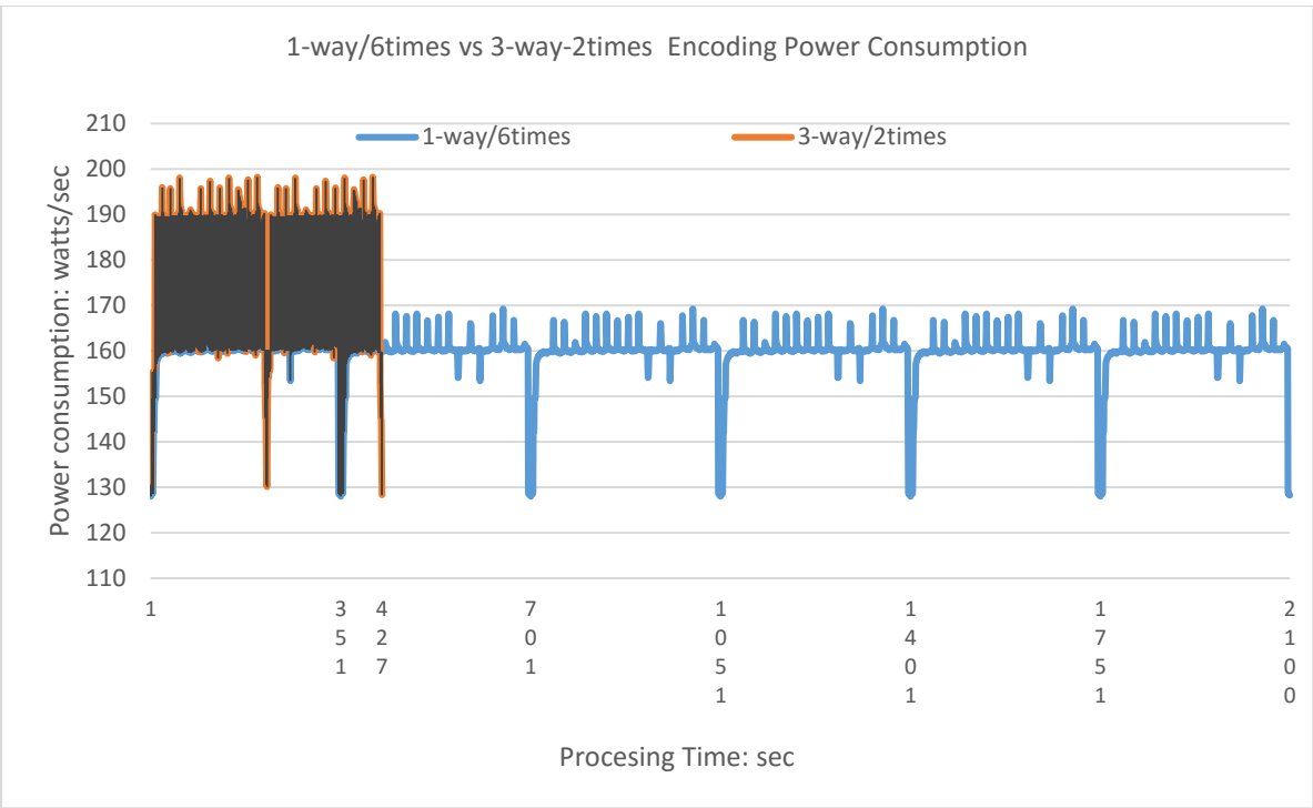
Figure-9b: Power consumption for processing six “34 GB” data sets -1 vs. 3 way parallel coding
