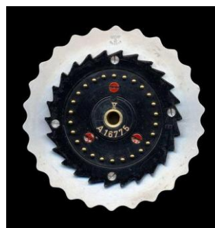
Fig. 2.3: Right side of rotor with 26 contact points.
