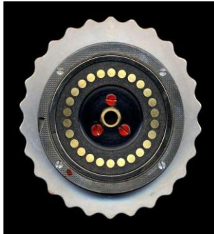
Fig. 2.4: Left side of rotor. The gray notched ring can be seen.
