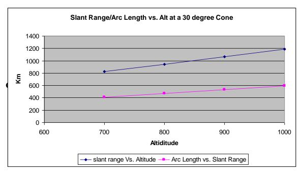
This graph represents the slant range and arc length at a satellites maximum footprint of 30 degrees. As shown the graph clearly increases as one goes up in altitude.
