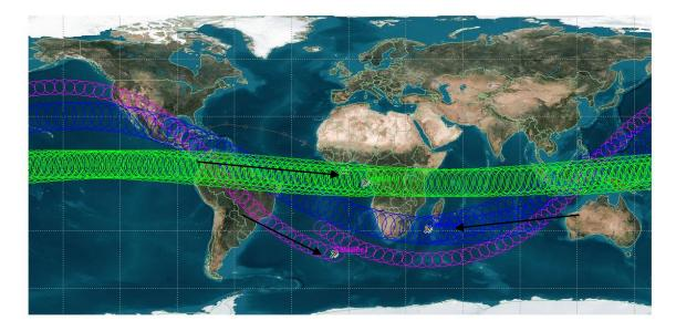
Our programming language was C++. With it, we were able to develop two tools to calculate the slant range and footprint of the satellites at various heights and angles. This allows anyone to simply input the altitude and angle desired to get back the footprint and slant range it would be at the specified settings.
