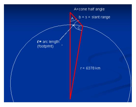
*CONE HALF ANGLE*: Angle created by the altitude and the slant range.
