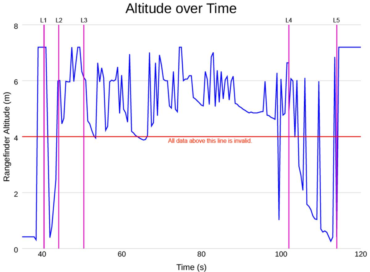
**Figure 6. The altitude measured by the sonar sensor over time during the failed autonomous flight.**
