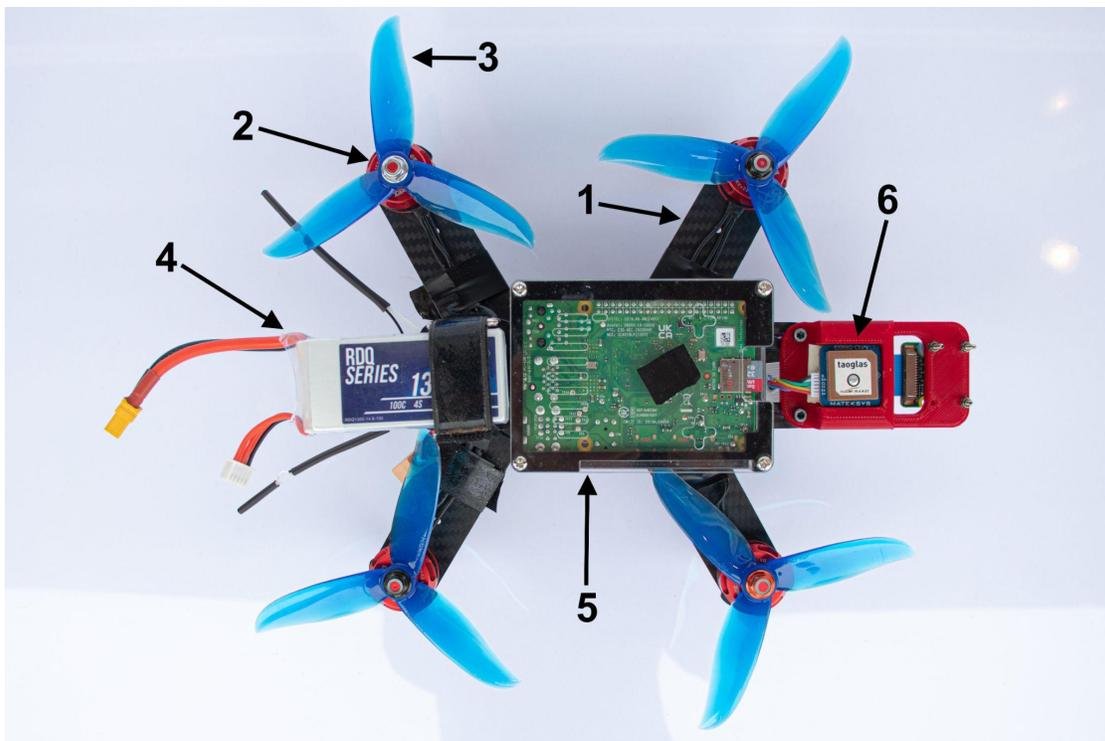
*Figure 2.1. A top view of the quadcopter with labeled components.*
