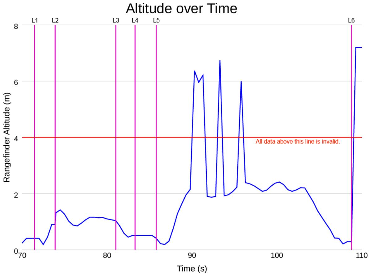
**Figure 8. The altitude measured by the sonar sensor over time during the successful autonomous flight.**
