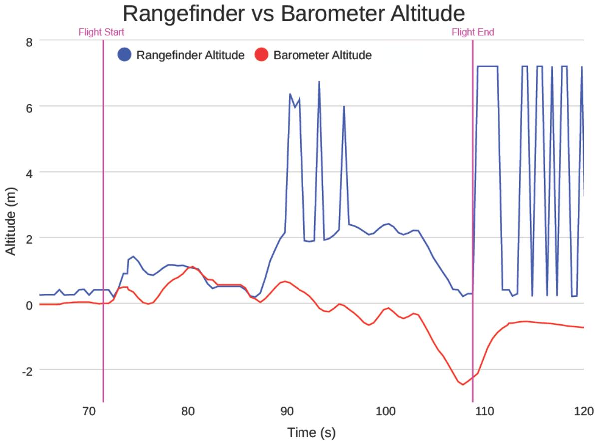
**Figure 9. The altitude measured by the sonar sensor compared with the altitude measured by the barometer.**
