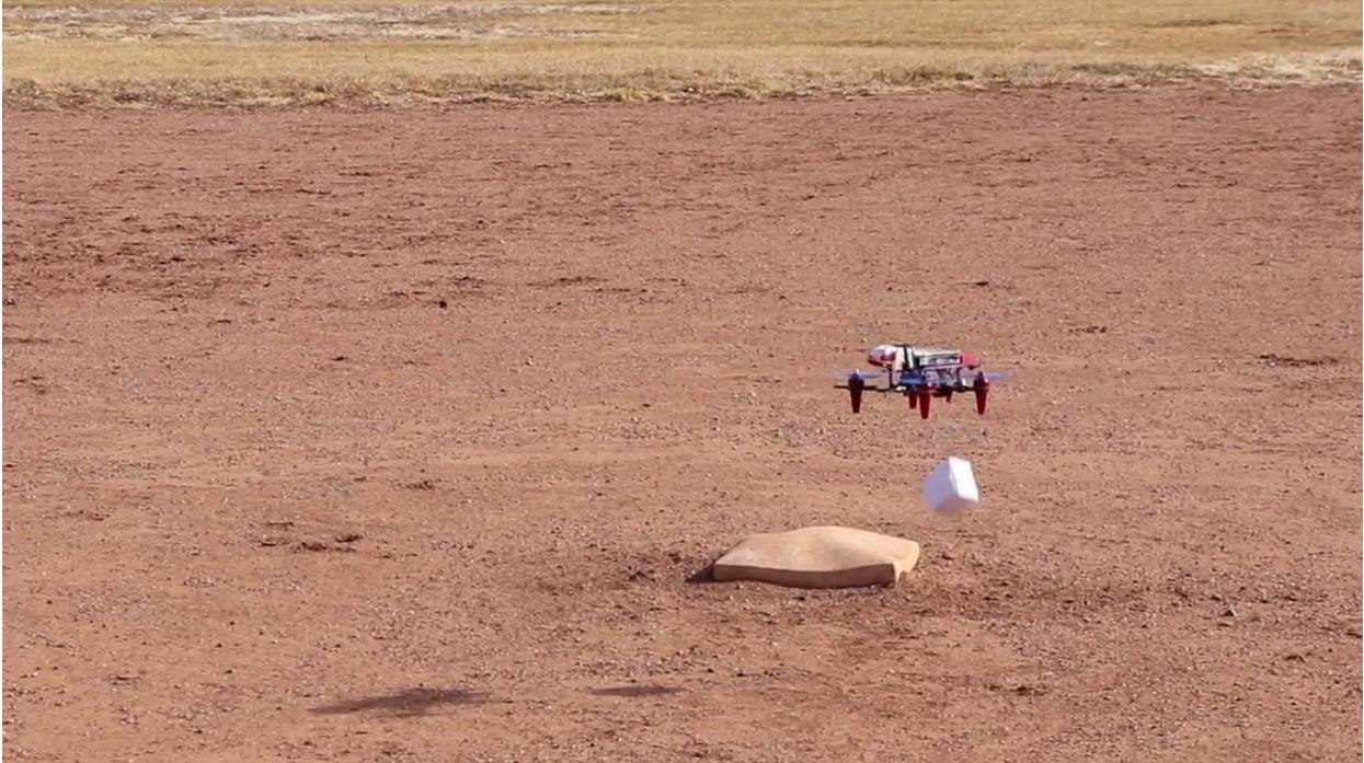
***Figure 7.2. The drone releases the package at a lower altitude.***
