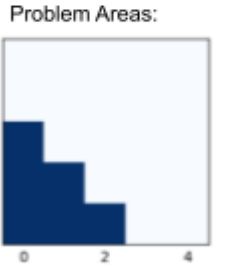
Figure 8 We expect to see 80cm as the maximum depth from the analytical tools for this geometry if the grid mesh perfectly approximated the elevation. 61.125 cm is expected for such a large grid pixel size.
