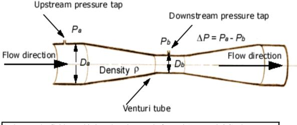
As long as the fluid speed is less than the speed of sound (V < mach 0.3), the <u>incompressible Bernoulli's</u> equation describes the flow. Applying this equation to a streamline traveling down the axis of the horizontal tube gives,
