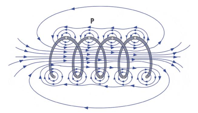
The lines of force are circular near the wire, but they become straight as we get to the middle point of the coil. Each segment of the coil is surrounded by similar magnetic lines of force. At the center of the coil, all the lines of force aid each other strengthening the magnetic field.
