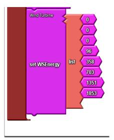
This is a variable which listed the energy output for wind speeds from 1-10 m/s.There is zero energy at less than 4 m/s.
