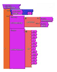
This is where the energy from the sun is counted. The first part is telling if the day is cloudy no energy is created. The next part is telling the average solar radiation each month.
