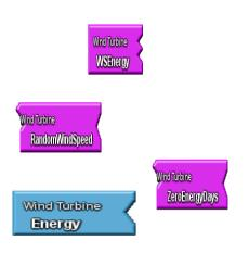
These are variables for the wind turbine. WSEnergy is a list variable for the energy generated at different wind speeds. RandomWindSpeed is the monthly wind speed plus or minus . ZeroEnergyDays is incremented whenever the wind is less than 4 m/s. Energy is an agent variable tracks the total energy per year.
