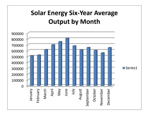
The monthly solar power output is highest in June and lowest in January. This graph shows the average monthly power in kWh.
